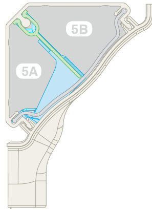
Cable fill #5: Divided Channel (power and data) with Low Profile Transition Insert.
