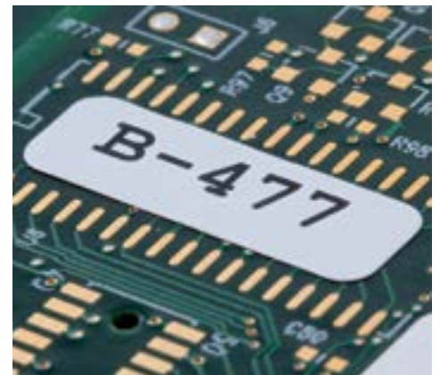
Electrostatic Dissipative Polyimide Label (B-477) Application
