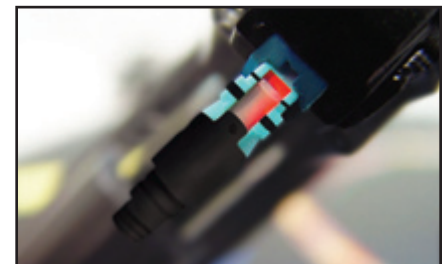
When used with the VFL, a light can be seen through the clear window on the connector body until a fiber has been properly terminated
