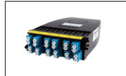
FC3U12LDMF1A, FX Ultra Cassette, OM3, 12 ports, MPO-12 (female), LC Duplex, Type-A ALT, Aqua adapters
