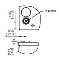
\*All dimensions in inches (mm). All dimensions are for reference only. Contact a C&D Representative for complete dimension information. NOTE: Batteries to be mounted with 0.5 in (1.25 cm) spacing minimum and free air ventilation.
