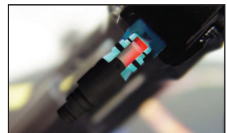
When used with the VFL, a light can be seen through the clear window on the connector body until a fiber has been properly terminated
