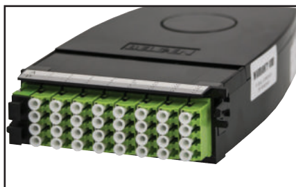
SCSH2116SLF, FX UHD Splitter Cassette, OS2, Dual 1x16 Splitter, SC/APC Upstream Ports, LC/APC Downstream Ports
