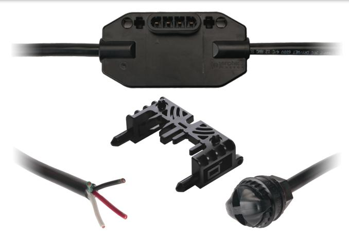
The Engage Cable is a continuous length of 12AWG cable with pre-installed connectors for Enphase Microinverters to plug into. The cable is handled like standard outdoor-rated electrical wire, allowing it to be cut, spliced and extended as needed.
