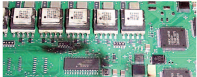
Internal Damage - PCB Destroyed By Overvoltage Surge
