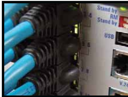
Hirschmann Industrial Ethernet Compact OpenRail Switch with RJ45 Industrial Ethernet connectors and stranded (Bonded-Pairs) TPE jacket.
