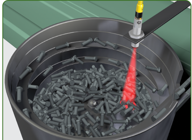
Feeder bowl application - A 42CM monitors bowl level to prevent component runout. This background suppression model ignores reflections from the bowl to accurately detect the components only.
