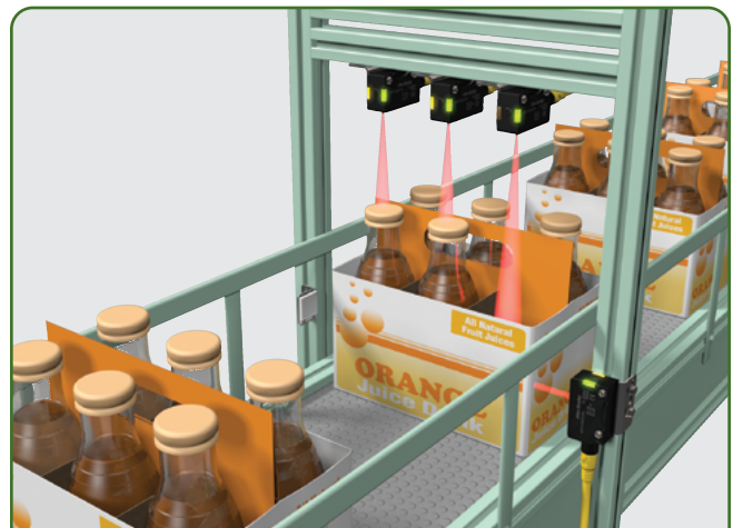
Bottling inspection - When the single 42JT LaserSight mounted on the side of the conveyor senses the bottle carton, it triggers the three standard VisiSights above to check for missing bottles.
