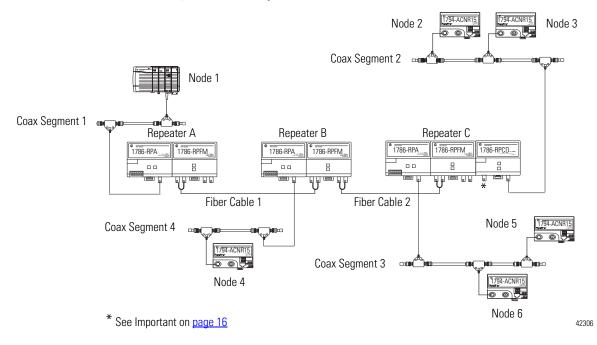
In <u>Figure 5</u>, the maximum number of fiber repeaters is 3, because a message from coax segment 1 to coax segment 2 travels through 3 repeaters in series (A, B, and C).
