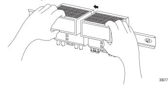
**IMPORTANT** Make certain that you secure the repeater adapter and repeater modules with DIN-rail anchors. If you do not, loss of communication or module damage may result.
