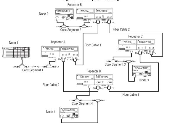
Figure 8 - Fiber Repeaters in a Ring
