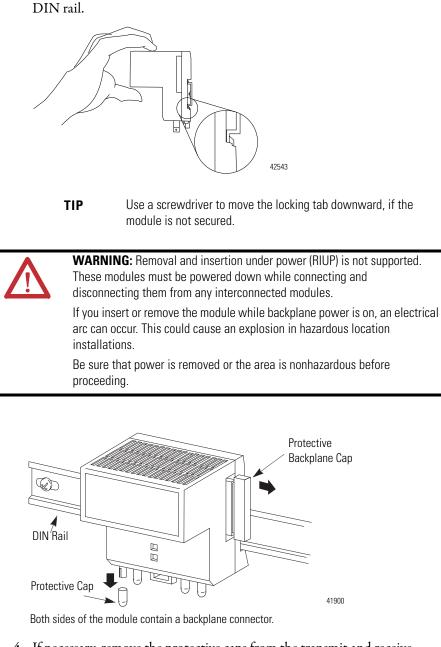
The locking tab should snap into position and lock the module to the DIN rail.
