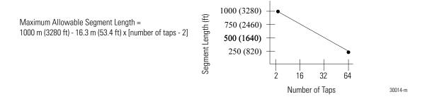
The data in Figure 11 assumes you are using standard low-loss coax. High-flex cable may not support the distance versus the number of taps due to the higher loss factor associated with high-flex designs.
