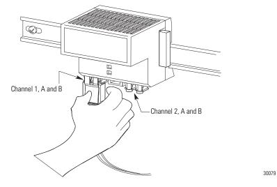
2. Hold down the latch and insert the other end of the duplex cable into another module by using either channel 1 or channel 2 of the other module.
