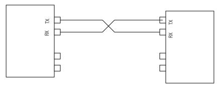
**TIP** Channels 1 and 2 on the module are identical. Channel 1 of a module can be connected to either channel of another module.
