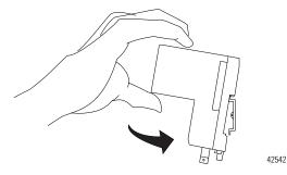
3. Press the module onto the DIN rail until flush.
