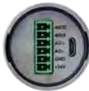
Thermalert 4.0 with 6-pin connector
