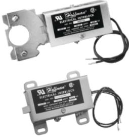
Provide positive internal safety lockout on electrical enclosures while the equipment is energized. When energized, these interlocks prevent the door handle from being turned to open the door.
