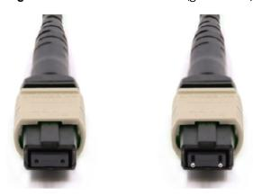
The 40G SR4 and 100G SR4 MPO transceiver modules use only cables with female MPO connectors, which have guide holes in the end face of the MPO connector (the transceiver has guide pins within the MPO receptacle).
