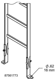
Secures ladder rack to floor, ceiling or wall. Made of steel with a painted or plated finish. One kit secures one ladder rack section. Requires surface mounting hardware (not included).
