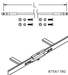
Fastens across splices to provide a secure ground between sections of ladder rack. Made of #6 AWG x 7 strand wire with green THW insulation and two-hole compression lugs mounted on each end. Includes fasteners.
