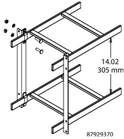
Allows stacking any width of ladder rack runways 12 in. (305 mm) above each other. Each kit contains two complete stacking brackets with all necessary hardware. Use one kit at least every 5 ft. (1.5 m). Brackets and fasteners made of plated steel.
