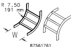
Provide a vertical change in direction. They are made of 1-1/2 in. x 3/8 in. (38 mm x 8 mm) tubular steel with a painted or plated finish. Cross members are welded on the inside (inside bends) or outside (outside bends) of the section. Connect to straight section with butt-splice kits. Designed for category 5e, 6, 6A and fiber optic cable.
