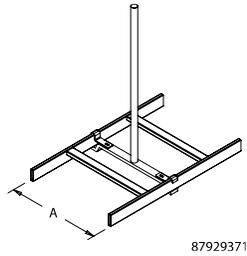
Threaded rod and bracket supports center of ladder rack from ceiling. Kit includes heavy-duty ladder rack cross member, 5/8-in. threaded rod, two J-bolts, protected sleeve and 5/8-in. nut. Use one kit at least every 5 ft. (1.5 m). Made of plated steel.
