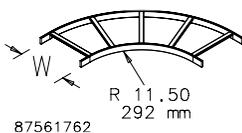
Provide a 90-degree horizontal change in cable runway direction. Made of 1-1/2 in. x 3/8 in. (38 mm x 8 mm) tubular steel with a painted or plated finish. Connect to straight sections with butt-splice kits. Designed for category 5e, 6, 6A and fiber optic cable.
