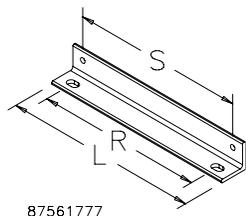
Supports ladder rack from wall or other flat surface. Made of 2-in. x 2-in. 10 gauge steel angle with painted or plated finish. Includes two J-bolts, nuts and screws.
