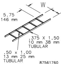
Supports cable on straight runs. Made of 1-1/2 in. x 3/8 in. (38 mm x 8 mm) 16 gauge tubular steel with a painted or plated finish. Nominal installed length is 10 ft. (3.05 m). Each section is 9 ft. 11-1/2 in. (3.03 m) long with cross members welded at 9-in. (229-mm) intervals.
