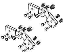
Provides a change in up-and-down direction of the cable runway. It can be adjusted to any angle from 0 to 90 degrees. Made of steel with a painted or plated finish. Each kit connects one ladder rack section to another. Includes mounting hardware.
