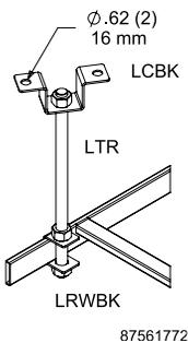
Supports ladder rack from ceiling. Components available separately or as a kit. Six-foot-long, 5/8-in. diameter rod is threaded for easy tension adjustment. Made of plated steel. Requires surface mounting hardware (not included).
