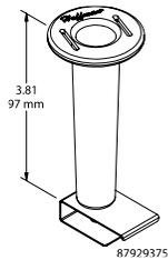
Spools separate cables to improve cable management and to control cable-to-cable distances. Spool and bracket attach to ladder rack cross member and can be located anywhere across the width. Kit includes ten 4-in.-tall spools, brackets and all necessary hardware. Spool made of black plastic and bracket made of plated steel.
