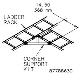
Provides additional support for 90-degree ladder rack junction. Made of steel with a painted or plated finish.
