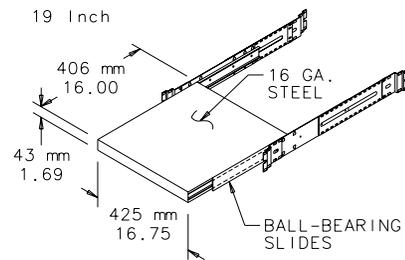
Pull-Out Shelves extend 17 in. (432 mm) on ball-bearing slides. 16 gauge pull-out shelf mounts to uprights in 19-in. electronic rack or 19-in. mini-rack using pull-out shelf bracket (EPSBKT) and has light-gray powder paint finish. Two screws captivate shelf to slides. 14 gauge steel pull-out shelf mounts between two pair of rack-mounting angles that have accessory mounting legs and has white finish. Plated mounting hardware is furnished.
