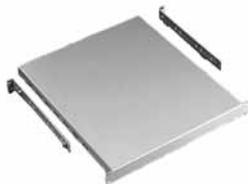
Mounts to front surface of front and back rack angles. Shelf is made of painted 14 gauge steel and the adjustable support brackets are clear-plated 12 gauge steel. Adjustable to fit multiple-depth enclosures or rack angle placement. Both solid and vented models available. Fits 19- or 23-in. rack spacing. Requires only 1U of rack space. Shelf has RAL 7035 light-gray textured or RAL 9005 black textured polyester powder paint finish.
