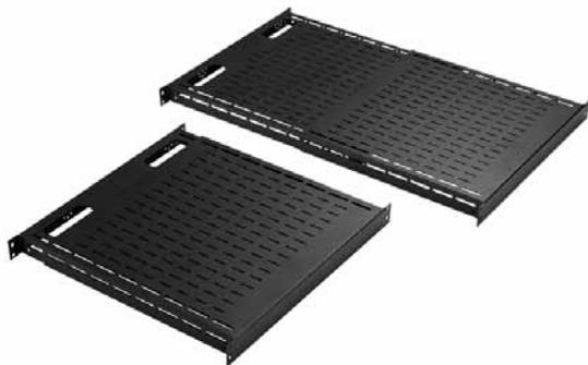
An easy-to-install tool-less vented 19-in. shelf. Mounts onto rack angles that have EIA-spaced square holes (.375 in.). Shelf slides open and provides a variable-sized, continuous surface for equipment. Back of shelf has oval cutouts for power and data cables. Accessory hole patterns at back of shelf fit small and large D-rings to help manage cable. Made of steel with a 150 lb. (68 kg) static load rating. Available with RAL 9005 black or RAL 7035 gray polyester powder coat finish.
