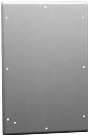
Constructed of 12 gauge steel and designed for use with 10 gauge and 12 gauge enclosures. Provides a removable cable egress and entry plate while maintaining UL/NEMA integrity of the enclosure. Gasket with pressure-sensitive adhesive is included to be applied after desired modifications are completed. Finish is ANSI 61 gray polyester powder paint. Maintains UL/NEMA Type 4 and Type 12 if properly installed in a Hoffman enclosure.
