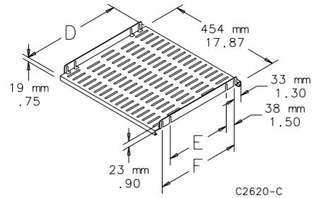
14 gauge steel fixed shelf has large ventilation slots in shelf surface. Mounts between two pair of rack mounting angles that have accessory mounting legs. Shelves have RAL 7035 light-gray polyester powder paint finish. Plated mounting hardware is furnished.
