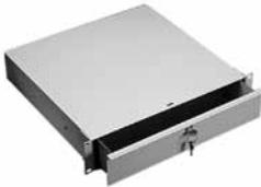
Steel drawer for 19-in. rack-angle mounting mounts to the front surface of the rack angles. Integral steel box contains the drawer and protects surrounding internal equipment. Extends 13 in. (330 mm) on ball bearing slides. Front includes handle and key lock. Finish is RAL 7035 textured light-gray polyester powder paint. Mounting hardware is included.
