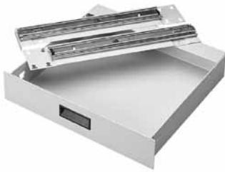
16 gauge steel drawer extends 17.00 in. (432 mm) on ball bearing slides. Drawer has polyester powder paint finish and recessed black pull handle. Drawers mount between two pair of rack-mounting angles that have accessory mounting legs. Includes provision for attaching a writing surface. Plated steel mounting hardware is furnished.
