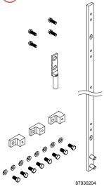
Mount vertically on rack, providing a convenient place to connect equipment grounds. Made of electrolytic tough-pitch 110 copper alloy. Kits include ground bar with compression lug for #2 wire, connection hardware, and mounting hardware.
