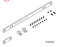
Mount horizontally on rack, providing a convenient place to connect equipment grounds. Made of electrolytic tough-pitch 110 copper alloy. Kits include ground bar with mounting hardware, eight #6-32 x 14 machine screws, and eight #6 ring terminals.
